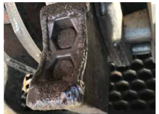
Minimal Damage to Insert/Tip
