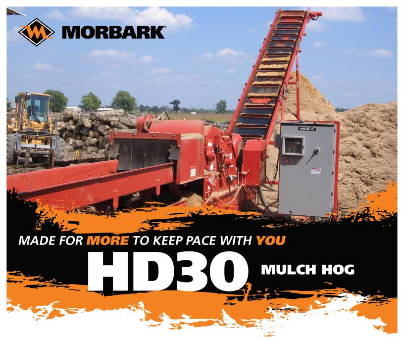
The **HD 30 Mulch Hog** converts low-value slabs, bark and sawmill waste into premium mulch products in a variety sizes depending on the screen used. At the heart of this machine is an electric- or diesel-powered hammermill. A large, double-door opening provides easy access to the mill for maintenance, and hammermill rods can be configured to be removed from either side. The stacking/discharge conveyor can be lengthened to allow top loading of vans.
