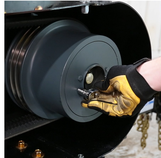
Reinstall the cover plate, bolts, and belt shield
