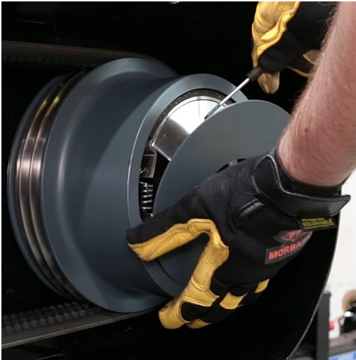
Remove cover plate to gain access to the ZeroClutch™
