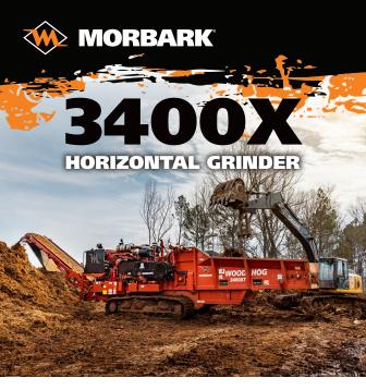
One of the most important features of the 3400X Wood Hog is its standard width of 8'6" (2.59 m), making it within the legal transport width in any country, no matter what engine is used. With 800 horsepower (596 kW), this model is ideal for a broad range of applications in a wide variety of markets worldwide. Like all of Morbark Wood Hogs, the 3400X also is available with electric power.
