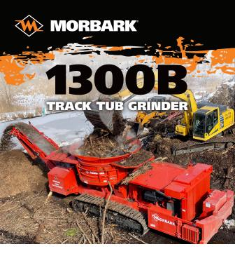
The Morbark 1300B Tub Grinder combines heavy-duty construction with the latest technology, including the Morbark Integrated Control System, which allows you to monitor critical machine parameters. With a full breakaway torque limiter system, hydraulic augers and a laser-cut hammer mill, the 1300B tub grinder is the most popular grinder on the market. The optional track undercarriage makes it easy to bring the grinder right to the material.
