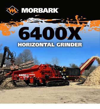
Ideal for processing wood waste, land clearing and storm debris into merchantable products, the 6400X Wood Hog's size allows it to be transported to nearly all domestic and international markets. The infeed bed is 24 inches (60.96 cm) longer than previous Morbark grinders in the 1,000-plus horsepower range and has sloped sides. This configuration improves operator sight lines for more efficient loading of material.
