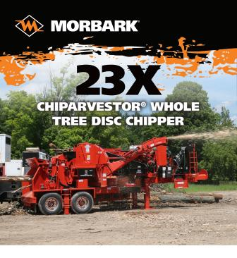
Morbark 23X Chiparvestor® whole tree chippers are built to last. The improved chipper hood design allows for better access to the disc during inspections and maintenance. Like the previous Model 23 Chiparvestors, the 23X uses a 75" (190.5 cm) diameter x 5" (12.7 cm) thick chipper disc to chip large volumes of wood, while the built-in dirt separator with deflector keeps the end product clean.
