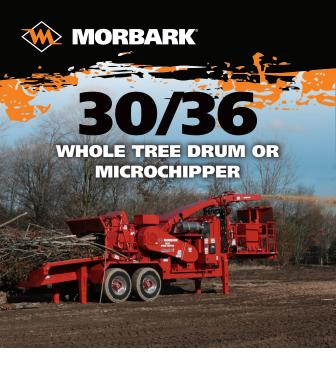
The Morbark 30/36 Whole Tree Drum Chipper's high production rate lowers operating costs by increasing fuel efficiency. The aggressive, sloped live floor feeding system, with two strands of durable WHD-120 chain and large top and bottom feedwheels, ensures positive feeding of material, including brushy tops and limbs. Morbark's Advantage 3 Drum produces more consistent chips, while the heat-treated, AR-450 steel drum skin provides longer wear life for lower replacement costs and less downtime.
