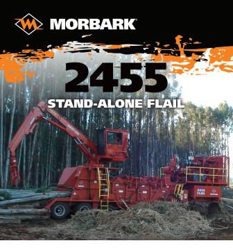
Whether used alone or in combination with a Morbark whole tree chipper to create a total fiber utilization system, the 2455 Stand-Alone Flail is built for maximized output. With three top feed rollers mounted on yoke assemblies, two stationary bottom feed rollers, and a bark discharge conveyor that folds for transport, this machine has many features perfect for whole tree chipping. The enclosed weatherized operator's cab with color-tinted safety glass helps protect the operator.
