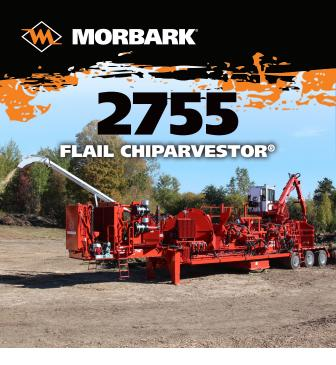
Offering three- or four-knife chipper disc options, the 2755 Flail Chiparvestor is ideal for some of your toughest jobs. A 27" (68.58 cm) diameter chipping capacity and lift capacity of 17,200 lb (7,800 kg) at 10' (3.05 m) make the 2755 one of the toughest machines for any job. The enclosed weatherized operator's cab is mounted on rubber shock absorbers and tilts hydraulically for transport and includes combination air conditioner/heater and six-way adjustable seat and joystick controls.
