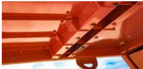
Removable infeed chain return floor, which allows excess material to fall away to minimize the wear on the floor, bed chain and inserts, particularly useful in land-clearing or other applications with dirty material.
