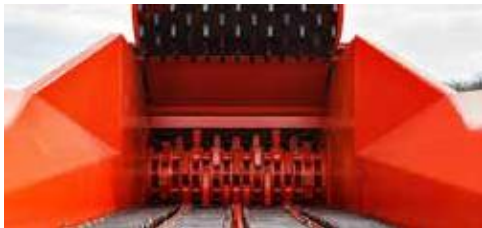
Large hammermill improves feeding characteristics, ease of maintenance and durability, while the configured hammermill pattern maximizes production output.
