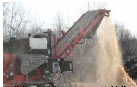
Optional folding conveyor with 14' 6" (4.42 m) discharge height
