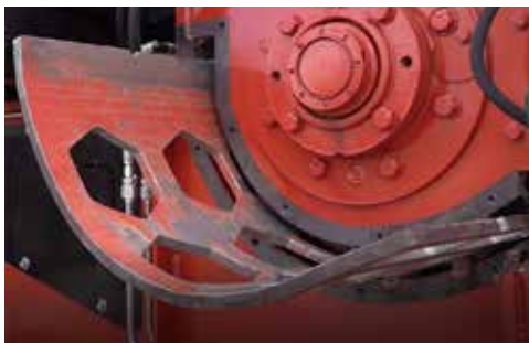
Single, side-load grate system and single side-load anvil allow for single-person removal.
