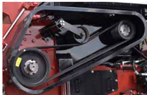
Adjustable backside flat idler allow the operator to adjust drive belt tensioning with no need to move the engine.
