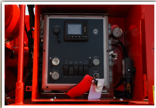
Morbark Integrated Control System The ultimate diagnostic system; monitors hydraulic pressures, temperatures, clutch systems and engine efficiency while automatically adjusting to maximize performance.
