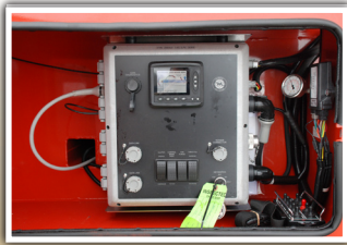
Morbark Integrated Control Systems Automatically adjusts feed rates, monitor pressures and feed wheel position to maximize production and engine efficiency.
